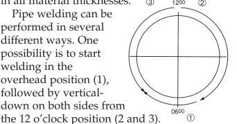
Another possibility is to start at the 7 o'clock position and weld vertical-up to the 11 o'clock position on both sides. This requires an inverter power source with a remote control.
