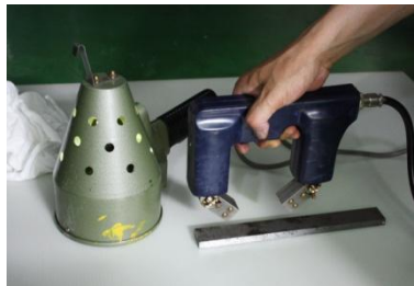
2. Forming the magnetizing current magnetic field
