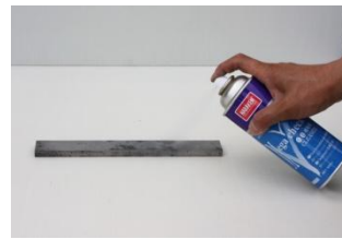
1. Cleaning of Testing Object
