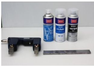
Testing Equipment & Magnetic particle Detecting Spray
