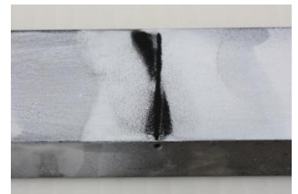
5. Examine the defective area with naked eye
