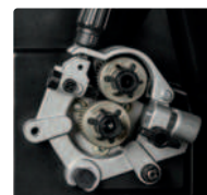
Heavy-duty aluminum two-drive-roll system
