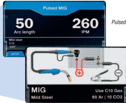
Connection screen for MIG process using C10 gas
