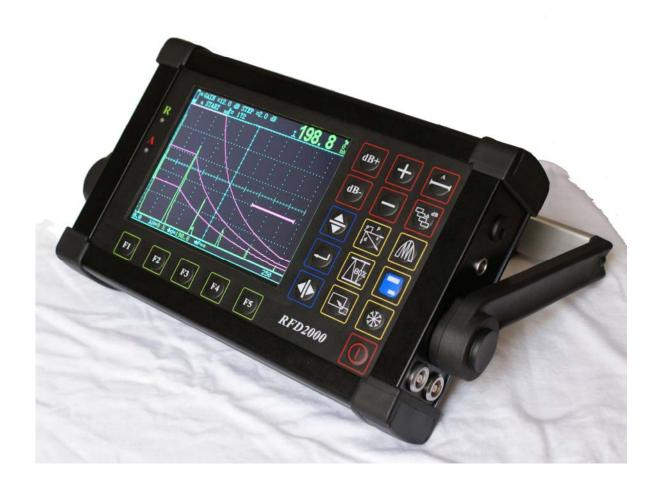
Automated calibration Automated gain Automated make video of test process and play DAC AVG B scan High-speed capture and very low noise Solid metal housing high contrast viewing of the waveform from bright Powerful pc software and reports can be export to excel
